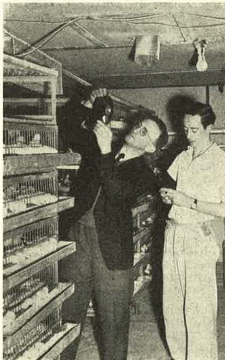
Heated hatchery. Mr. R. Nadenbousch (L), engineer, tests air velocity in an air conditioned room at this Bentleigh farm.
